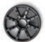
Plastic Support after Hammering (The form of the 8 supporting blocks will become altered to fit with the screw)
